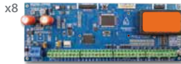
P/N - CM705PB 8/16 Universal LAN Zone Expander PWA Only F.01U.275.880
